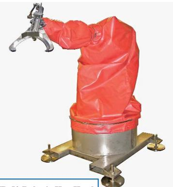
The Jarvis Model JR-50 Robotic Hog Head Dropper for continuous head dropping operations on the kill floor.
